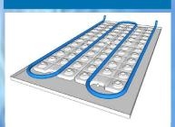
It's easy to upgrade these passive cooling systems into an active chilled ceiling. This greatly improves the flexibility of a conventional HVAC system. Should, for any reason the HVAC machinery fails the frozen PCM modules offer an uninterruptable emergency relief cooling system giving the facility maintenance team an opportunity to react.
