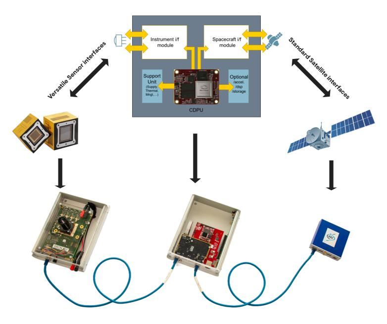
With the support from the Netherlands Institute for Space Research (SRON) and Airbus NL, we have built a demonstrator integrating an Engineering Model of the SPEXone instrument together with the CDPU; the CDPU controls the SPEXone instrument and performs the real-time image processing of the SPEXone data (both over SpaceWire using CCSDS packet handling).
