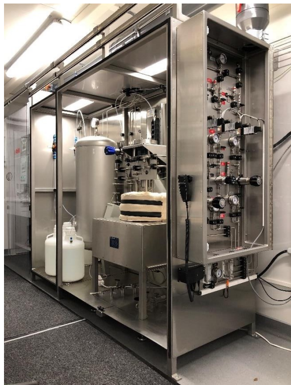
The autoclave (middle), gas filling station (right) and H 2 S capture system (left)
