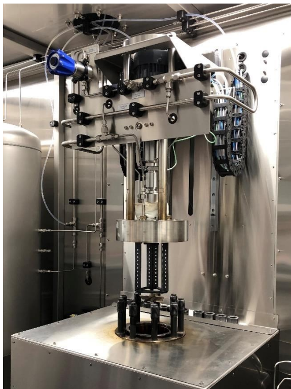
The autoclave with the lid opened before installation of test samples in the sample holder
