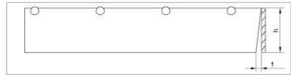
Fig. 23. Bevel of cutting of load bearing flat bars in relation to the transverse bar
