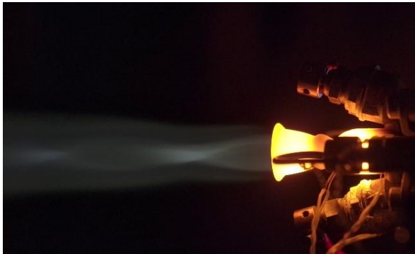
HyNOx-1 thruster during hot fire
