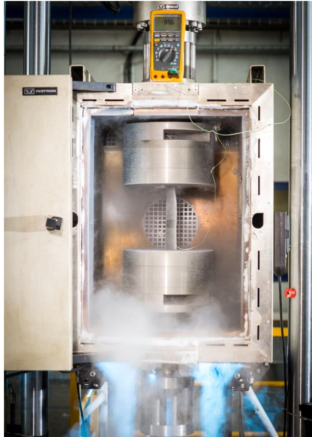
Fatigue test at cryogenic temperature
