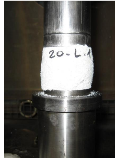
Compressive test on a ceramic specimen
