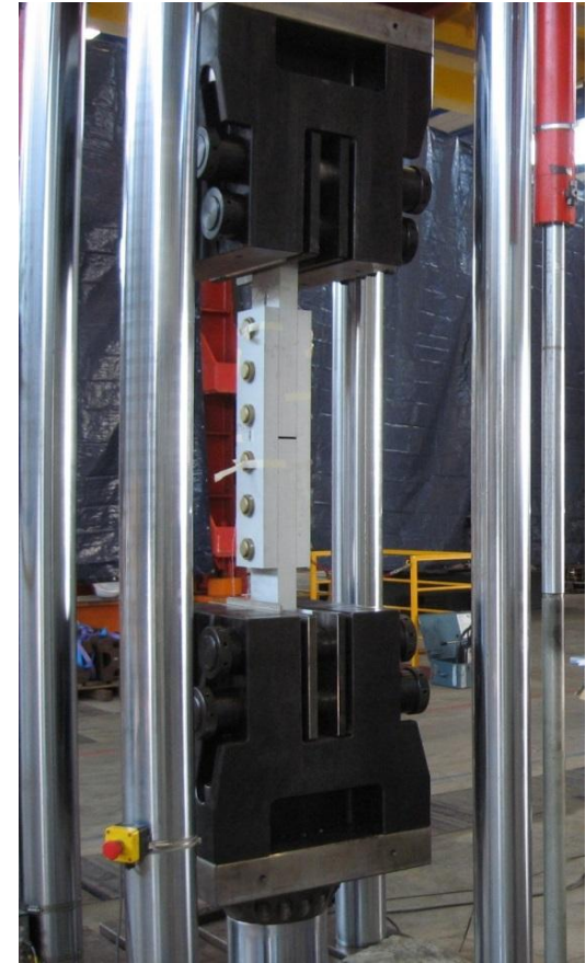
Fatigue test on composite-metal assembly
