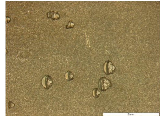
Macrograph of pitting corrosion specimen
