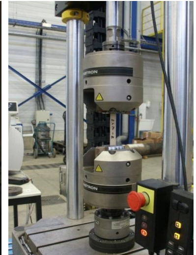
Tensile test on a 50 \mu\text{m} thickness glass fiber specimen
