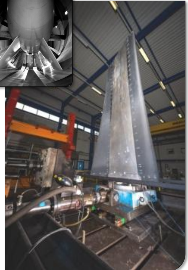
Vibration test on a metallic-composite wind tunnel blade for ONERA
