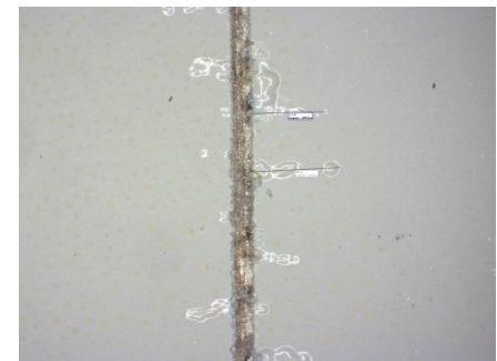
Macrograph of a filiform corrosion specimen after test
