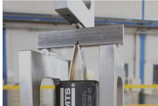
Crack growth rate test on SENB Specimen
