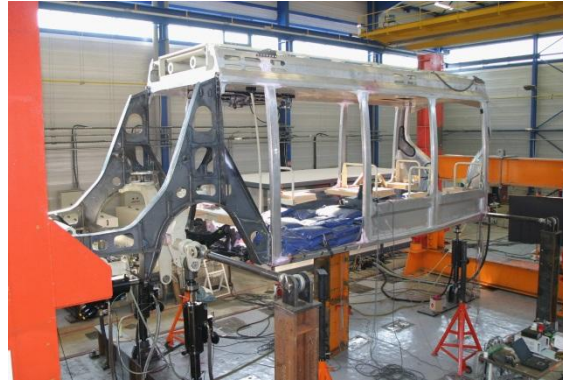
Fatigue test on a railway structure
