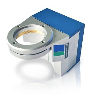
The objective positioner MIPOS 800 SG is a long travel positioning and scanning system, based on a high stiffness flex hinge piezo design. It offers a travel range of up to 800  $\mu m$  in open-loop operation, and 650  $\mu m$  in closed-loop.
