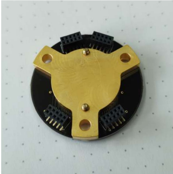
Sample Carrier Pad 40 bottom view
