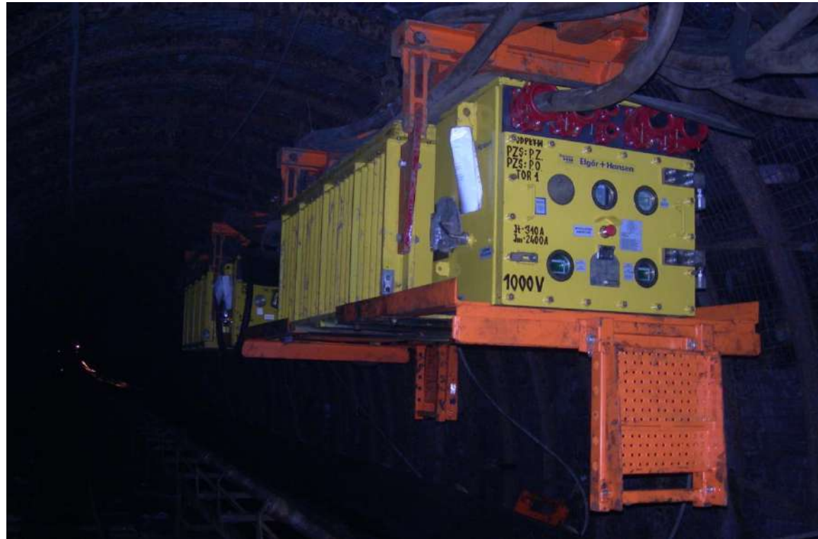
Transformer on double-carriage set type 20-60.4 (load capacity 11980kg) in KWK Zofiówka, Jastrzębie-Zdrój.
