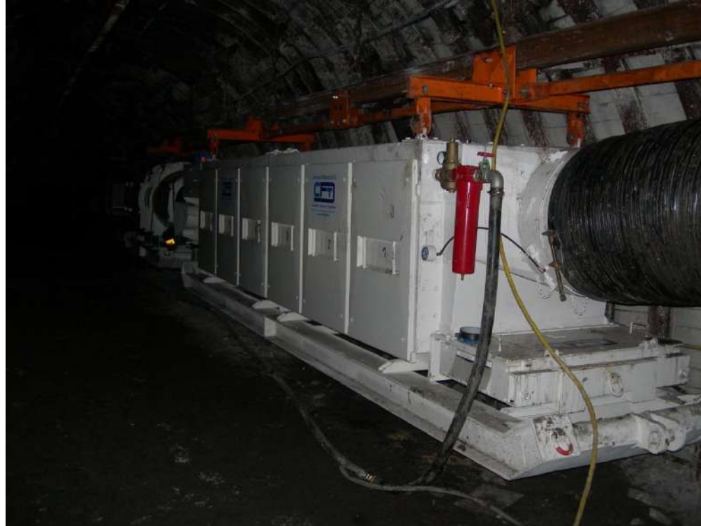
Dust removal device on carriages with extension arm type 20-364 (load capacity 2x4000kg) in ZG Sobieski, Jaworzno.
