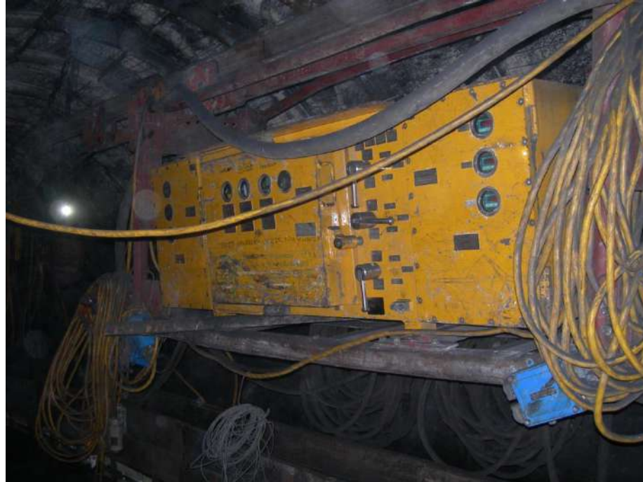
Compact station on pallet type 20-316 (load capacity 3000kg) in KWK Marcel-Marklowice, Radlin.
