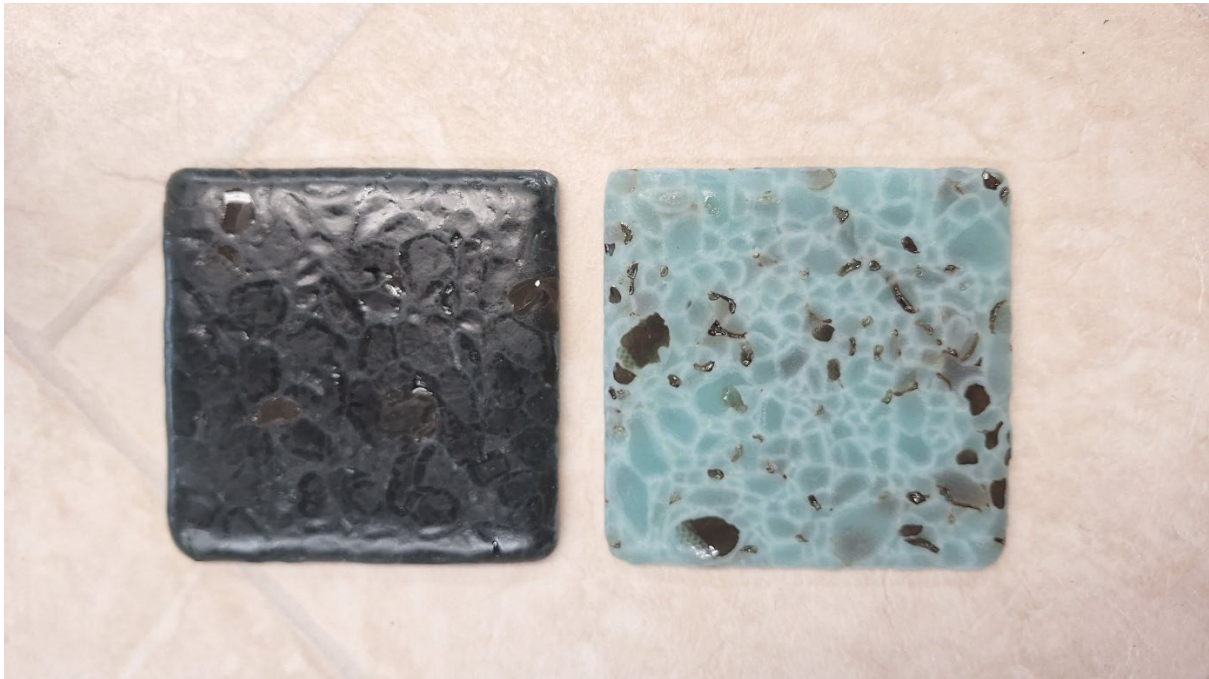
Figure 8, Test specimens: Black privacy glass on the left and green-tinted glass with distinctive black edge paint on the right.
