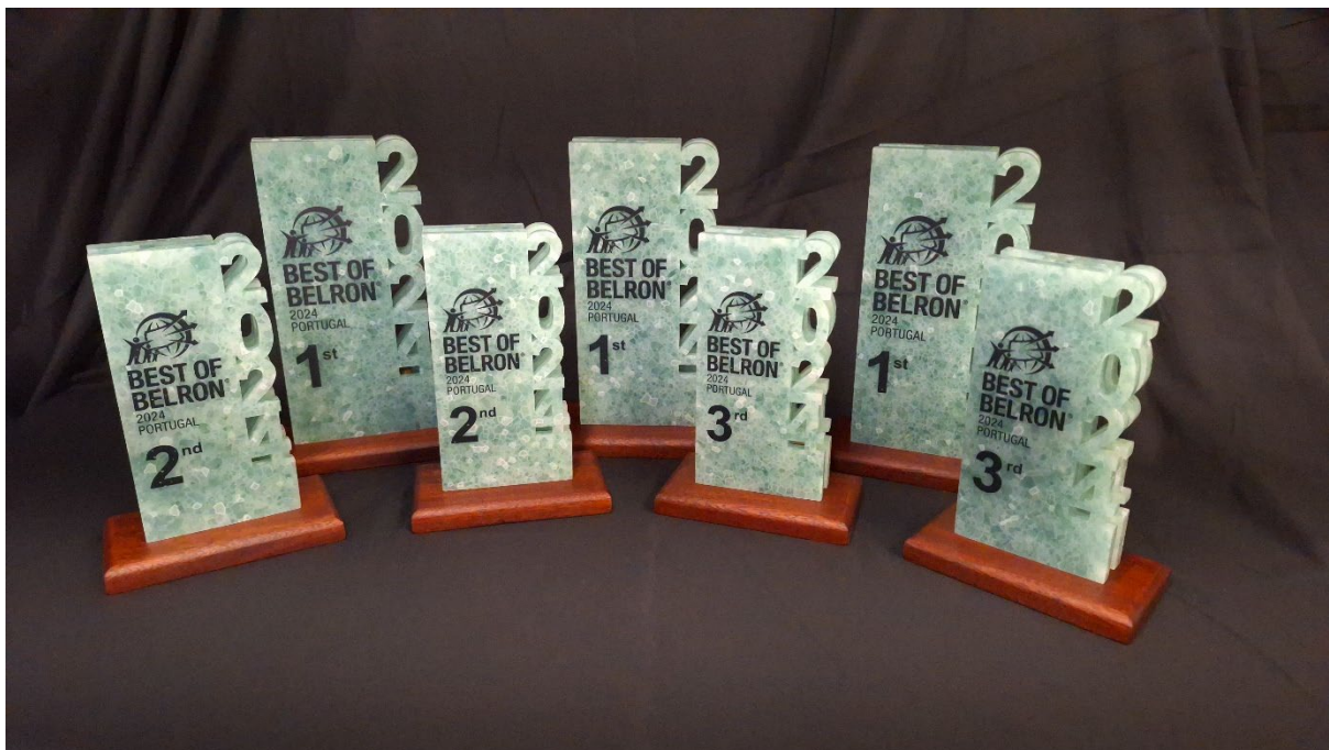
Figure 4, Award trophies: Waterjet cut, polished, printed, and layered on a wooden stand.
