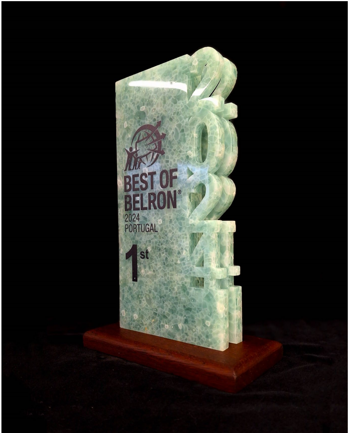
Figure 2, Award trophy: Waterjet cut, polished, printed, and layered on a wooden stand. Dimensions: 280mm H x 140mm W, featuring three layers of 12mm thick glass.
