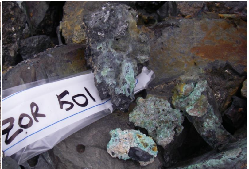
Sample of slag ZOR501 contains 0.15% Co and 2.9% Cu , 0.09% Ba , 1% S (elevated cobalt and copper contents remain in slag because in historic smelting process only half of cobalt and copper has been extracted).
