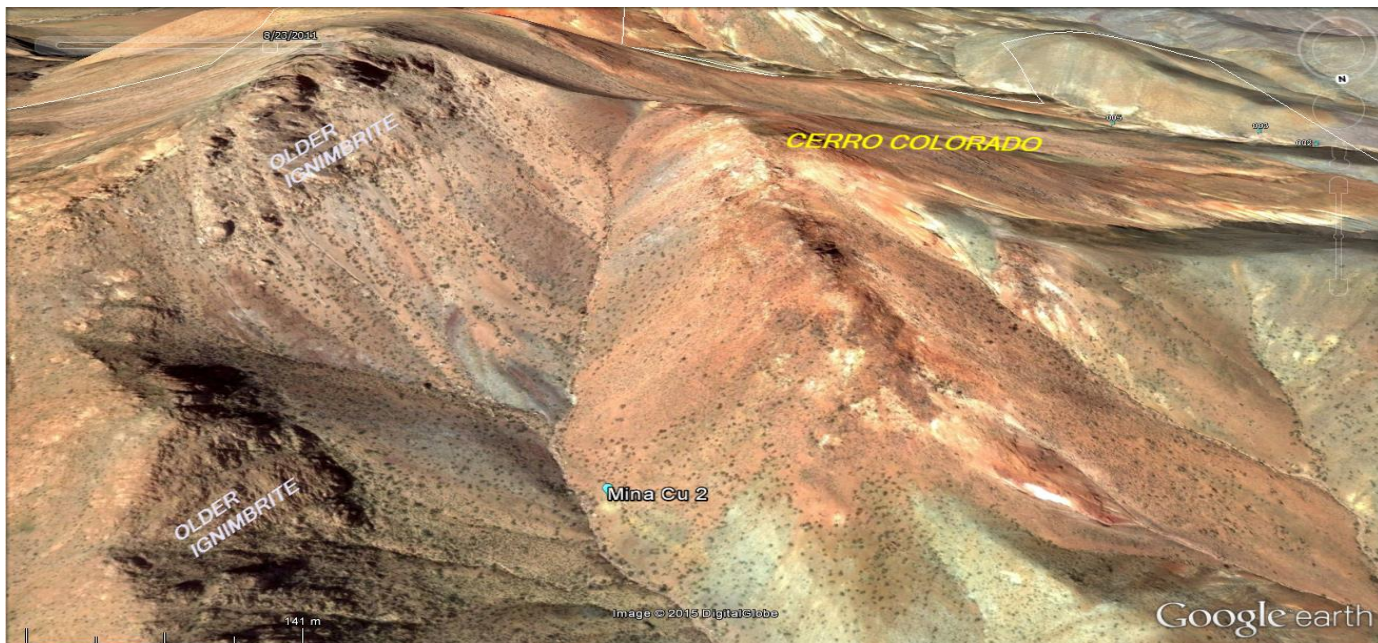
Panoramic Google Earth views (looking S and SW) – Southern Cerro Colorado ‘leached capping’ with a historic mine marked “Mina Cu 2” located in the valley where the ‘leached capping’ has been eroded to expose oxidised ‘secondary enriched zone’.
