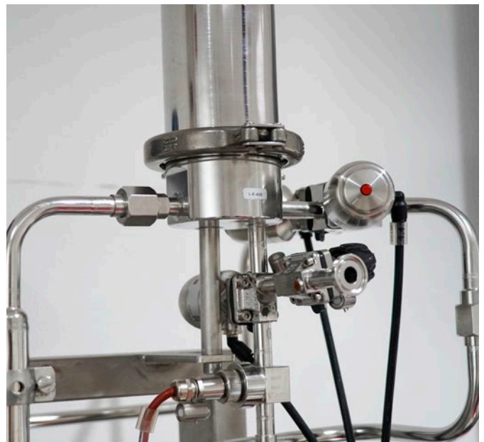
Conventional construction of a filter base with process valves welded on
