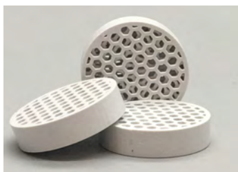
Examples of possible complex geometries for SOC devices or catalytic reactors.
