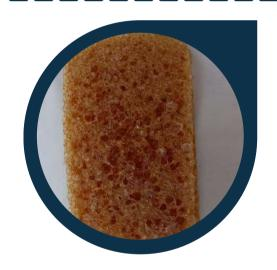
HYDRO-PUR is a porous foam that has a honeycomb-type structure and allows it to house plant germination (by dripping) or insect nesting in its macroporous structure. Although it does not have thermal or acoustic properties, it is a foam designed for integration into natural ecosystems in urban environments.
