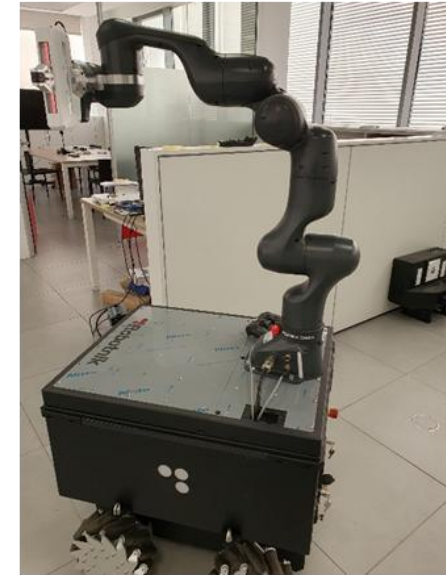
mobile cobot on omniwheel base
