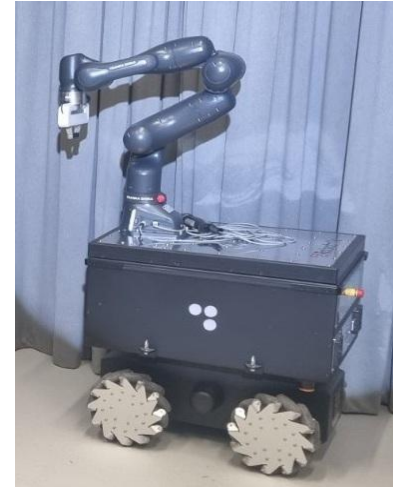
mobile cobot (Franka Research III on Robotnik omniwheel base)
