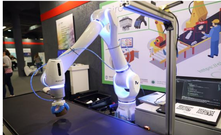
computer-vision and AI for handling moving objects of arbitrary shape
