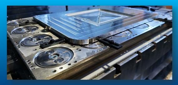
A) D75 mm discs provide suction and support
