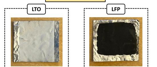
The initial trial on depositing battery materials on Al foil sprayed through Low Power Plasma Spray
