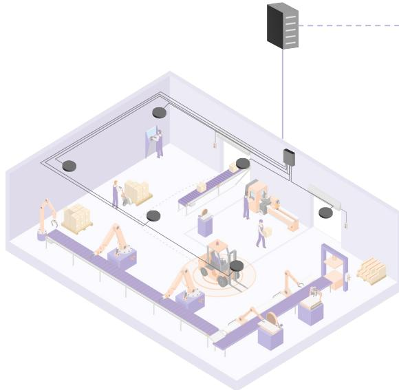
1 We install digital displays at each material location along the line, and/or paper labels integrated with the e-Kanban service.
