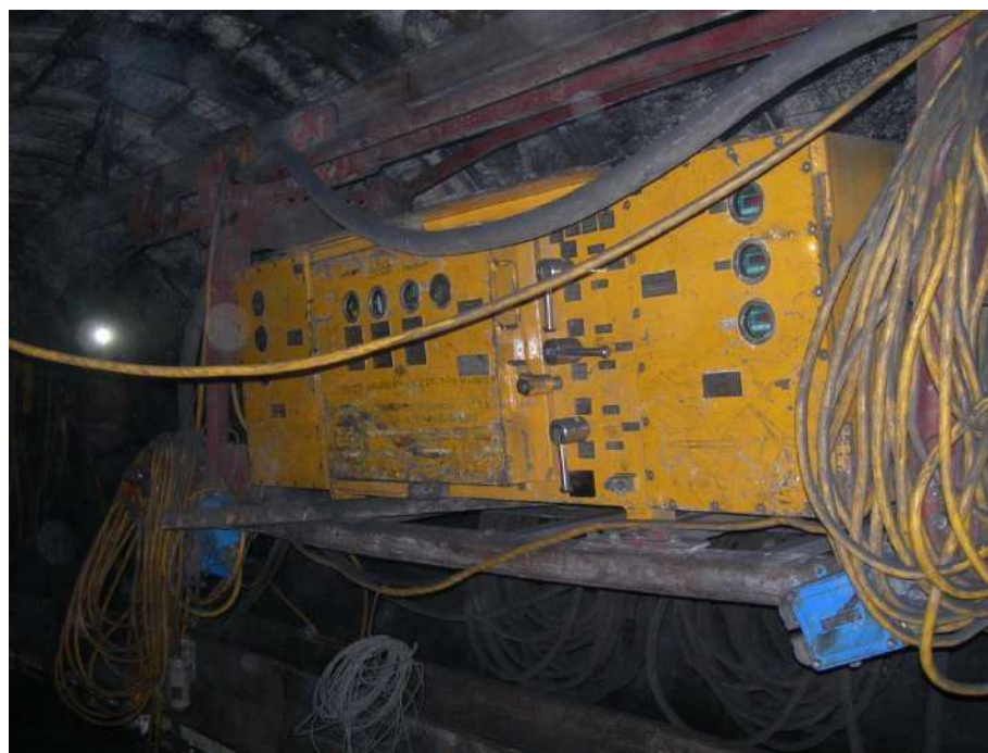
Compact station on pallet type 20-316 (load capacity 3000kg) in KWK Marcel-Marklowice, Radlin.
