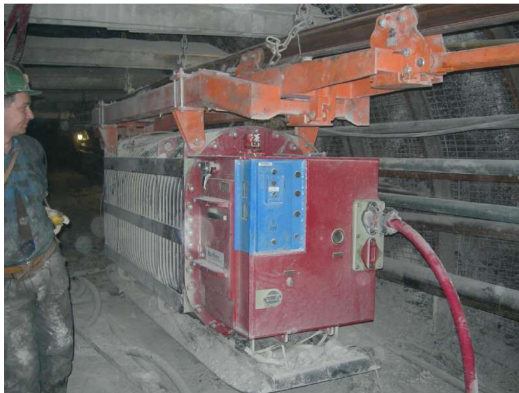
Transformer on frame type 20-325 (load capacity 10600kg) in KWK Staszic, Katowice.
