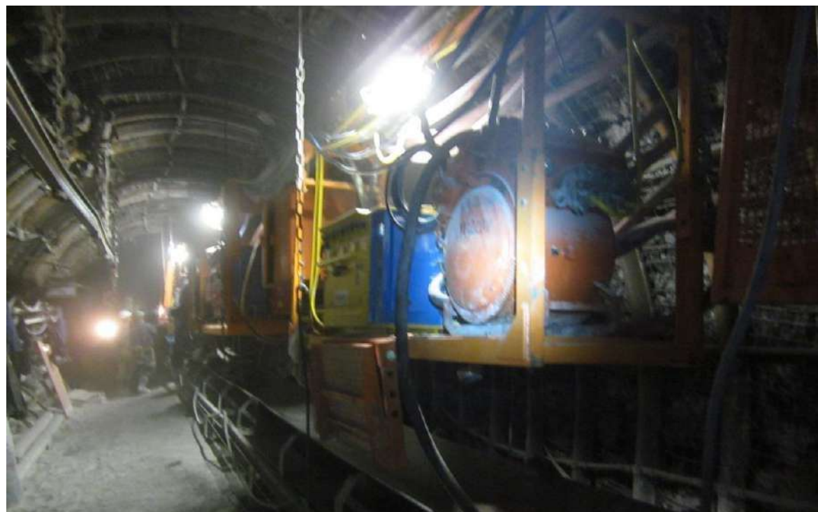
Power switch on pallet type 1-488 (load capacity 1000kg) in PG Silesia, Katowice.
