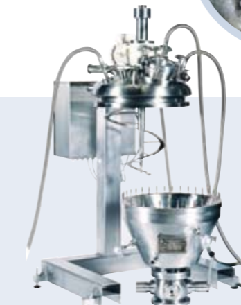
VRIECO-NAUTA CT 50 VERTICAL RIBBON DRYER
