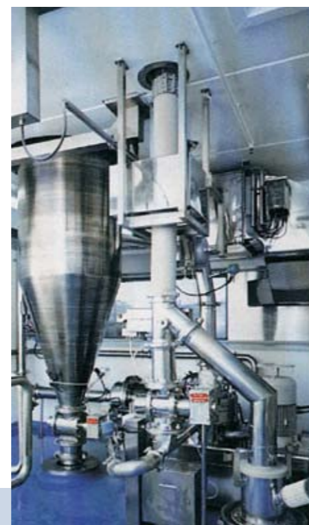
MULTI-PROCESSING MILLING SYSTEM INCORPORATING ALPINE 70 ZPS AND 140 AFG
