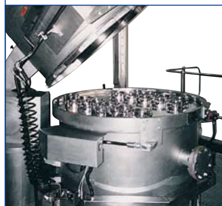
SPECIAL BAG PLATE FOR MIKROPUL PHARMA FILTER
