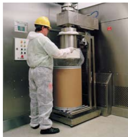
STOTT FILLING AND WEIGHING SYSTEM WITHIN A VITALAIR DOWNFLOW RECIRCULATION BOOTH
