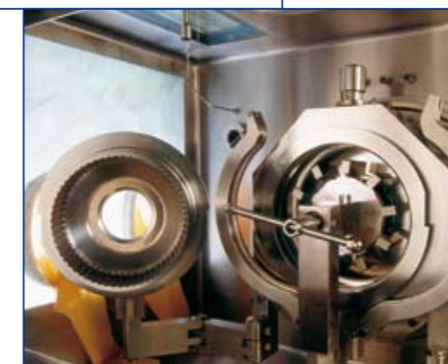
FELXIBLE ISOLATOR (OEL < 10 \mu\text{g}/\text{m}^3 ) WITH 50 AS IN PVDF
