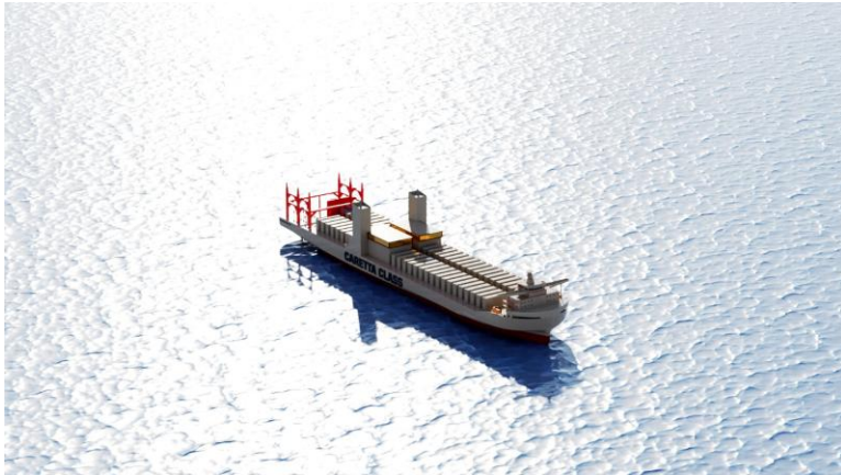
Caretta Class (BESS) Capacity: 500-1,000 MWh
