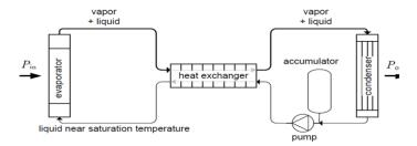
The vapor then flows to a condenser where it is condensed back into liquid.
