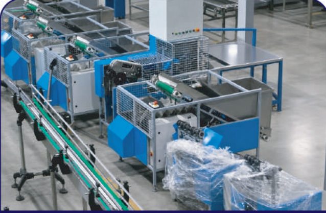
STİX ÇUBUK KONTROL MAKİNESİ STICK ICE CREAM STICK INSPECTION MACHINE
