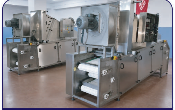
SOĞUTMA VE TOZ ALMA TÜNELİ COOLING & DUST REMOVAL TUNNEL
