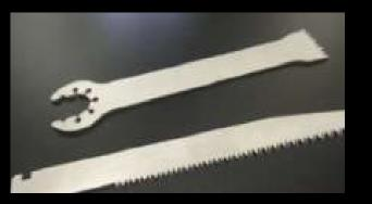
Shaped hole and sheet metal laser machining (tolerance + / - 0,01mm)
