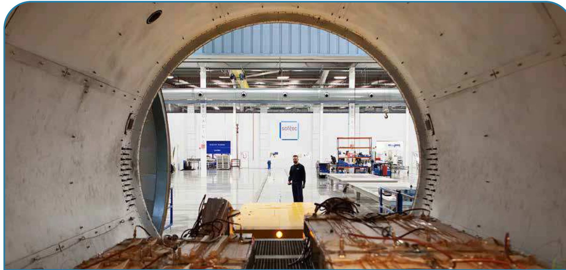
2 AUTOCLAVES. 4 x 1 6 m . / 1 3 x 5 2 f t (DxL)
