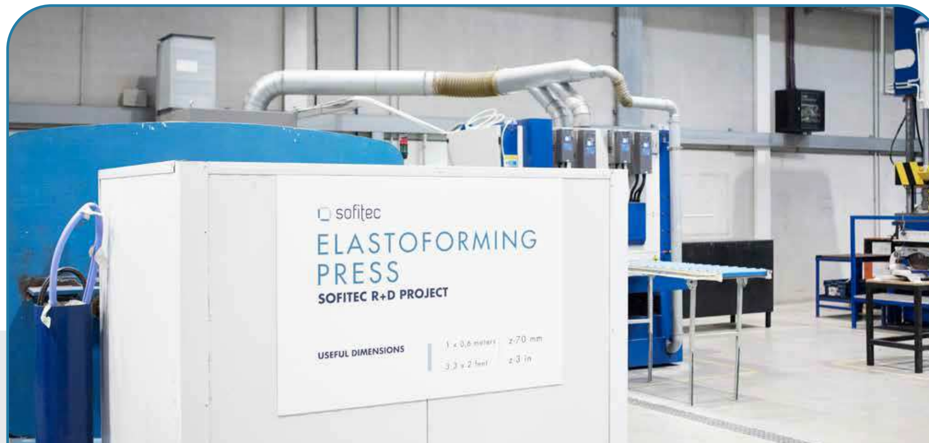
ELASTOFORMING PRESS 800x500x55 m m./ 3 1.5x19.7x2.17 in . | 300 bar
