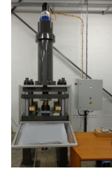
Creep test bench
