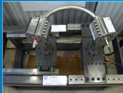
Pure bending test bench (+/-90°)
