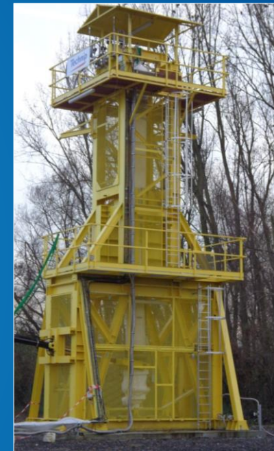
Cryogenic-bending fatigue test bench (250 kN)
