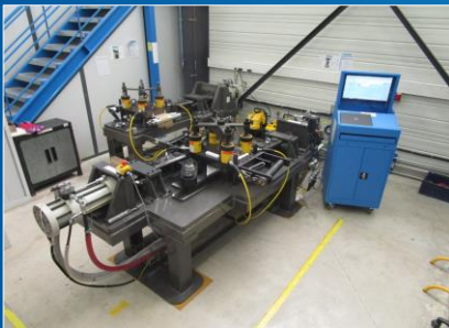
Compressive/shear combined test bench (300 bar/400kN)
