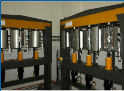
Multi-post fatigue test bench (-20°C/+80°C, +/-10kN)
