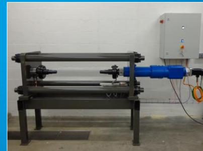
Creep test benches (up to 600 kN)
