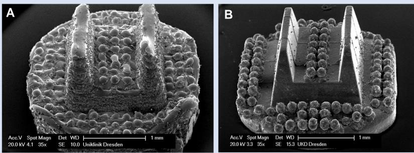
The brackets were covered with polymer (Trogamid) by injection molding. The coating of the brackets was almost complete, at around 98%. Only the bracket base showed minor coating defects, which can be neglected.
