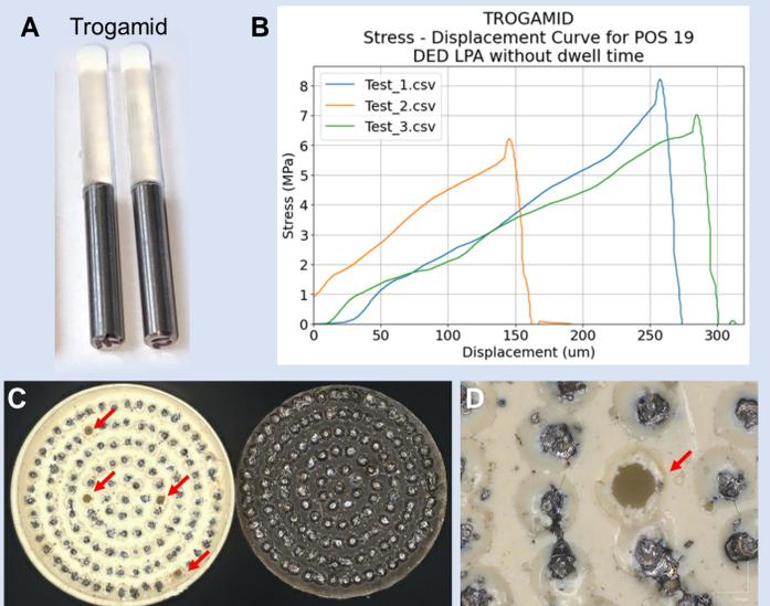
No damage to the Trogamid coating was observed under simulated clinical conditions [simulated ageing processes (B) and repeated cleaning with toothbrushes (C)] compared to the initial state of the polymer-metal brackets (A).
