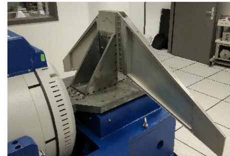
Design and vibration test – prototype of wing shape
