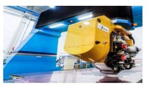
ATL Prepreg Gantry - MTorres Tape width 75 to 300mm.
