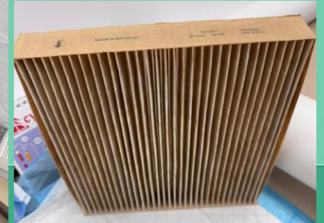
Volvo Filter Coated with 10% OliQuell
