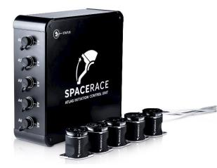
The ICU (Initiation Control Unit) is an advanced solution designed for easy initiation of hold-down and release actuators in ground test campaigns of space mechanisms. With intuitive control software, configuration of release scenarios becomes simple - achieved within seconds with a few clicks on your PC. This user-friendly unit ensures synchronized activation of up to 5 actuators via current pulse with millisecond precision.
