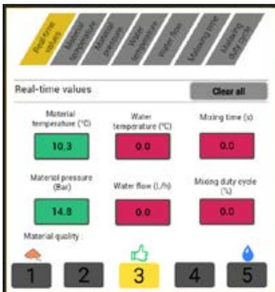
Pumping system data acquisition directly displayed on MaxiPrinter control interface. Contact us for more details.
