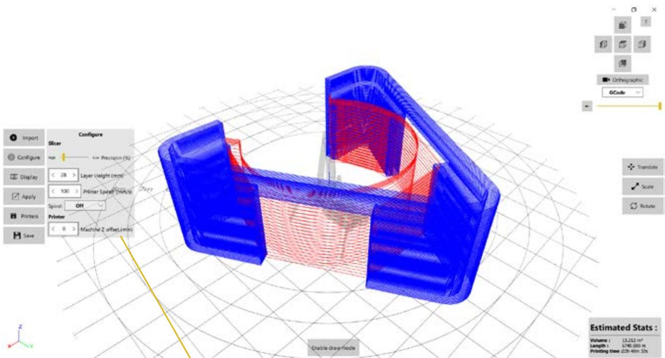
Configuration of the slicing mode, (spiralized or standard) layer height, nozzle speed, curve precision.
