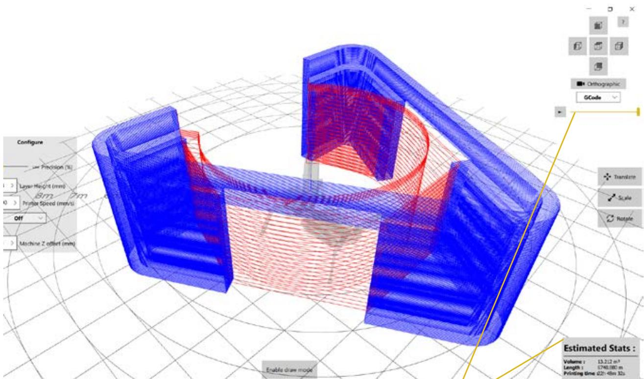
Visualization of G-code, trajectories with and without extrusions. Estimation of the amount of material needed and the printing time.
