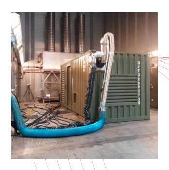
We can simulate solar heat up to 950 W/m² and our testing facility is equipped with infrared thermal cameras and sensors to monitor the behaviour of the test objects. We test your equipment thoroughly, to provide you quality and reliability assurance or detailed insights into potentially hidden deficiencies when operating in extreme weather conditions.
