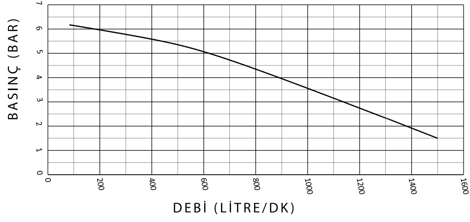
P1 BENZİN MOTOPOMP PERFORMANS EĞRİSİ
