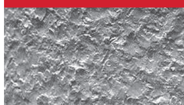
Fig. 10-12 SEM Photo of Single Peen Surface Finish
