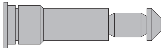
Fig. 6-1 Brake Pin Schematic
