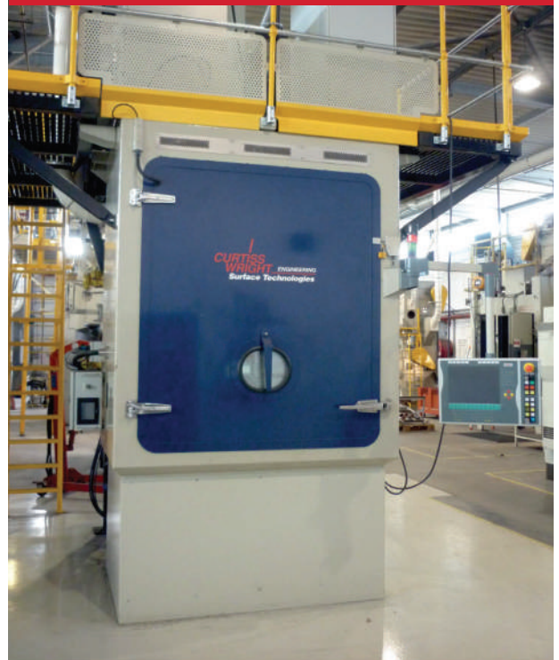
Fig. 11-10B Multi-Nozzle Computer Monitored Shot Peening Machine
