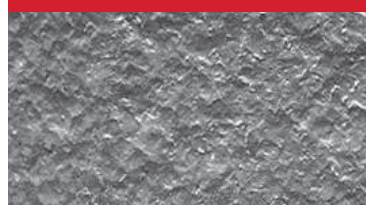
Fig. 10-13 SEM Photo of Dual Peen Surface Finish
