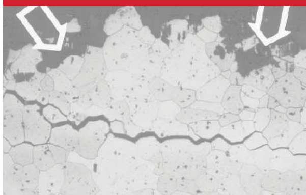
Fig. 8-3B Primary and Secondary Cracking from Intergranular Corrosion
