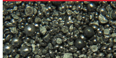
Fig. 11-3B Poor Quality Shot Peening Media
