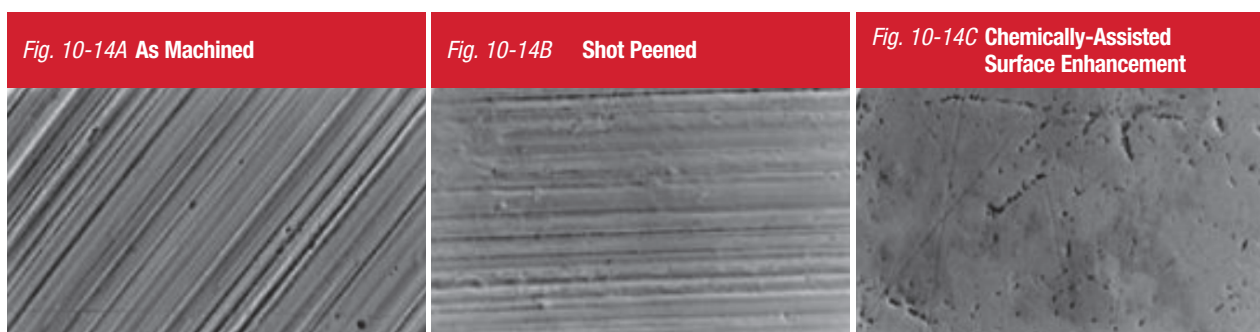
Figures 10-14A to 10-14C show typical surfaces at a 30x magnification
