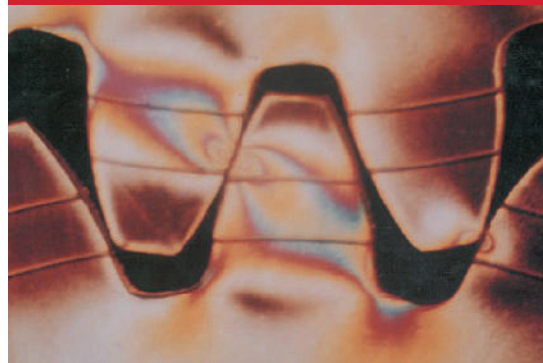
Fig. 4-3 Polarized View of Applied Gear Stresses
