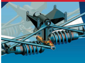
Fig. 5-2 Compression Spring Assembly
