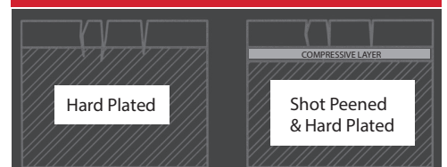
Fig. 3-4 Compressive Stress Resists Micro-Crack Growth
