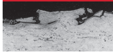
Fig. 11-2B Typical Surface from Proper Media
