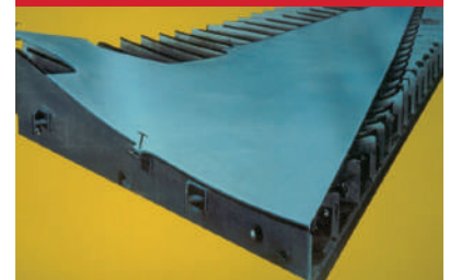
Fig. 10-2 Checking Fixture for Verifying Peen Forming of Wingskin
