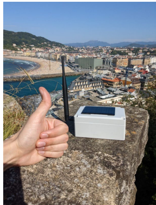
Embedded solar panel powered Isurlog LoRa outstation at the Urgull mountain in San Sebastian (Spain), linked to ISURKI's headquarters based LoRaWAN gateway through 13 km of hilly terrain. ↑ ↓
