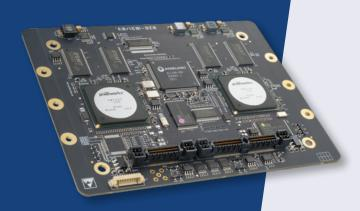
The MFD 21 board is a penta-processor video control board for managing multifunction displays with resolutions up to FHD. It features advanced multi-vision functionalities: PiP, PoP, zooming, panning, and digital freeze frame. The controller can manage up to 24 video signals in formats: DVI/HDMI, VGA, CVBS, SDI-3G, allowing the simultaneous display of 4 selected sources.
