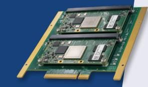
The VIN 338-HELIX is a dual-processor LCD controller for managing multifunction displays with resolutions up to XGA. Designed to equip avionics display systems, it offers advanced functions for video signal management, including; Picture-in-Picture (PIP) and Picture-on-Picture (POP), with adjustable sizes and positions, digital freeze frame, dynamic On-Screen Text, and video enhancement.
