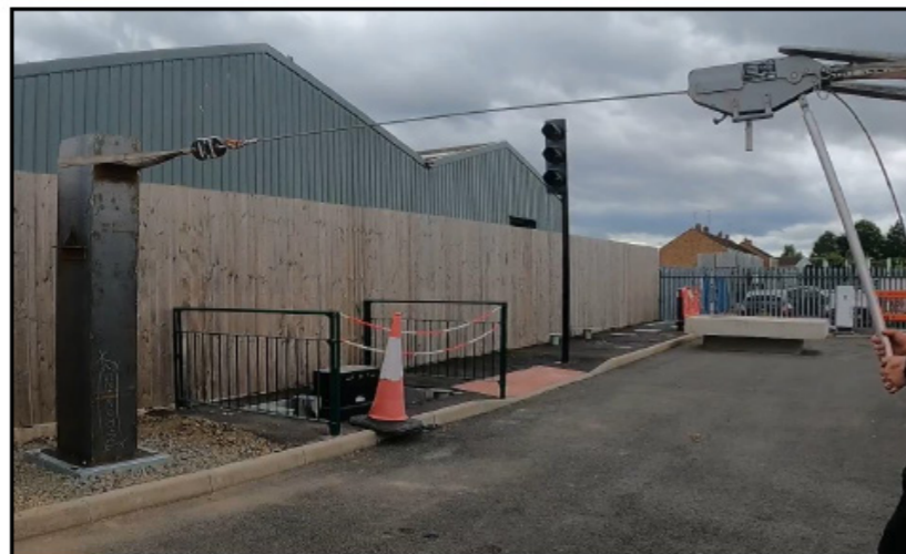
Sling attached around charger connected to digital force gauge and crank lever mechanism
