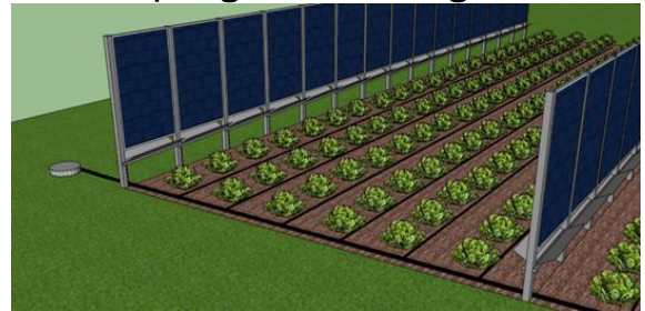
Fig 2: Agrivoltaic infrastructure with drip irrigation
