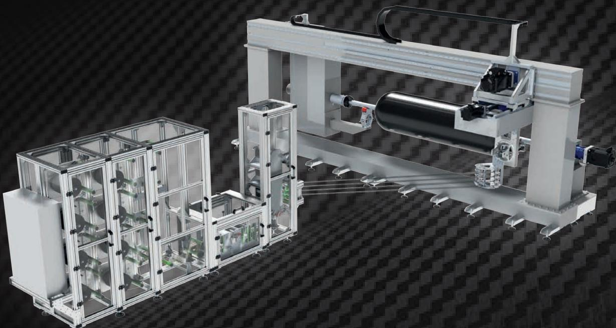
**APOLLO** is designed for the manufacturing of CPV tank, with a creel of 8-spool system, it combines wet winding and tow prep winding in one machine.
