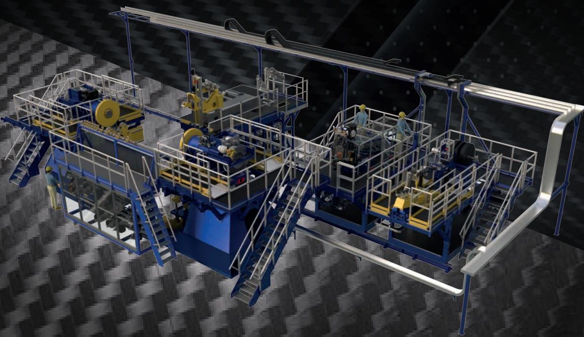
**ZEUS** is a cartesian machine to produce composite structure for aerospace applications.
