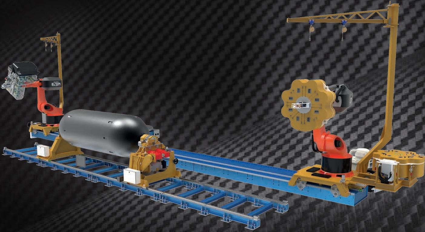
**ARES** is the result of the fusion between **EFESTO** + **ATENA** + **robotic milling technology** in one machine for the production of composite cryogenic vessels for aerospace applications (type IV and type V).
