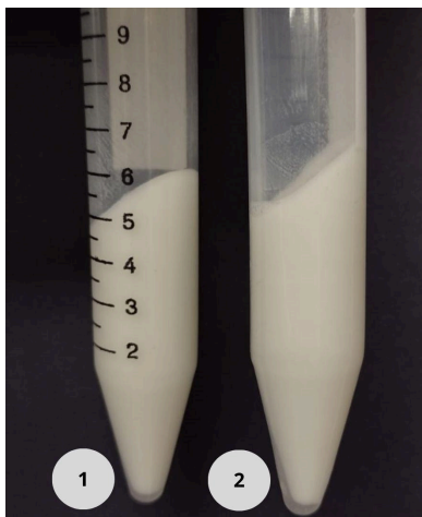
Figure 4 - Samples containing 5% SSO after 1: centrifuge and 2: thermal stress tests.
