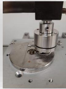
C. Plane vs plane contact mode
