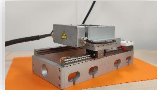
D. Tribo-tests at high temperature in the reciprocating configuration
