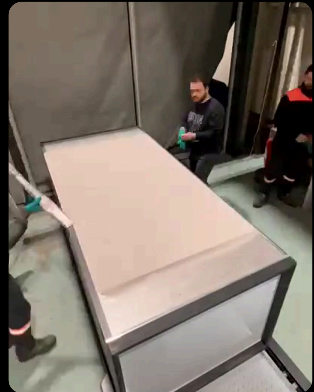
Depowdering process of produced sand molds
