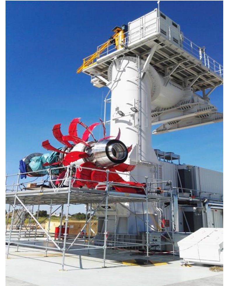
Contra Rotating Open Rotor Full scale test rig in Istres
