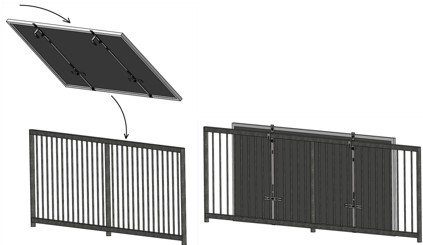
FIG.7 Installation of the structure on the railing
