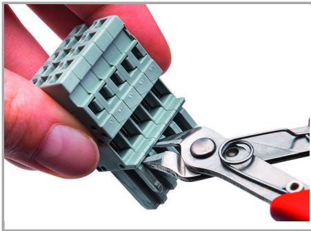
Coding a female plug by removing coding finger(s) via cutting tool. Do not remove the first and last coding fingers or use an additional locking lever.
