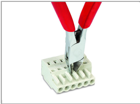
Coding a female connector – removing coding finger(s).
