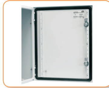
The doors in enclosures for heights of 400 mm and more, are equipped with vertical reinforcements with mounting holes spaced 25 mm.
