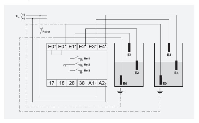
Functions: 2u2, 2d2 2 containers, 1 probe connected to E1 and E2, 1 probe connected to E3 and E4
