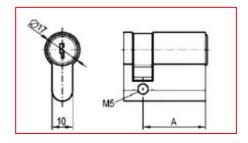
Profile half cylinder according to DIN 18252 (EN 1303)
